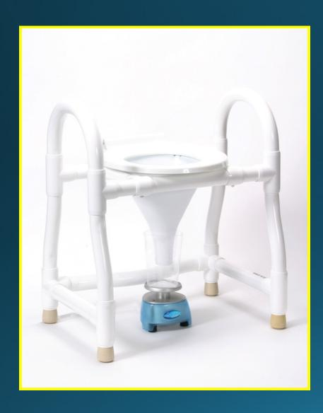
Rate of change of the weight of the voided volume converted into flow rate
